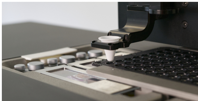
Gentle, automated laser microdissection of single cells, followed by precise transfer to a 96-well plate using CellCut HT.
