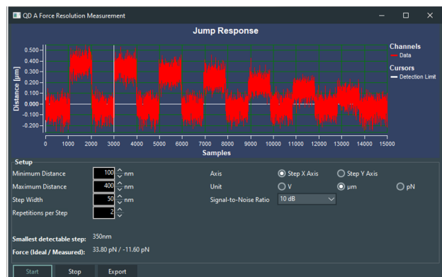
Fig. 7: Jumping experiments to verify the voltage-displacement calibration.
