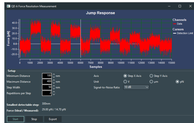
Fig. 9: Jumping experiments to verify the displacement-stiffness calibration.
