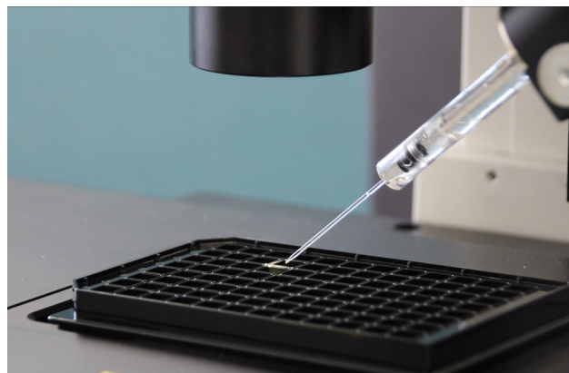
The MMI 3D CellRobot for rapid and ultra-precise recognition, acquisition and deposition of single or rare cells in suspension in a 96-well format.
