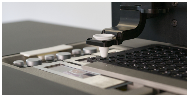
Gentle, automated laser microdissection of single cells, followed by precise transfer to a 96-well plate using CellRobot.
