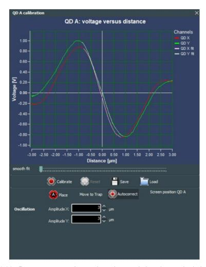
**Figure 6.26:** Response curve of a quadrant detector in imaging mode during calibration
