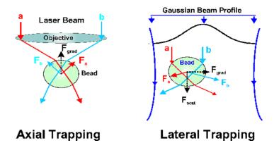
Figure 4.2: Forces exerted during trapping of particles
