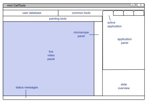
Figure 5.1: Structure of the mmi CellTools user interface
