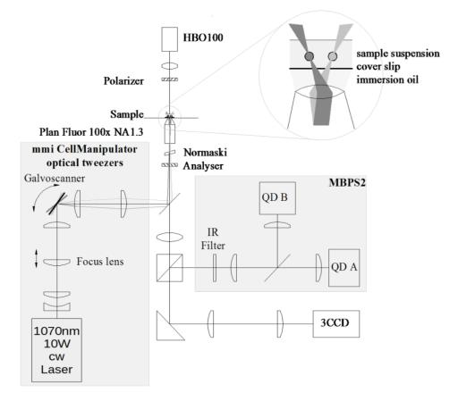
**Figure 4.1:** Setup of the mmi CellManipulator with a one level optical trap, a standard inverted scientific microscope with DIC illumination and the microbead position sensor.
