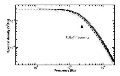
**Figure 6.18:** *Power spectrum obtained from the Brownian motion of a trapped particle*
