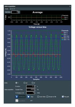
**Figure 6.25:** Response curve of a quadrant detector when correctly adjusted, Y oscillation
