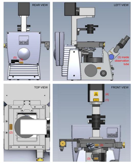
Figure 1.2: Positions of laser safety labels in mmi CellManipulator
