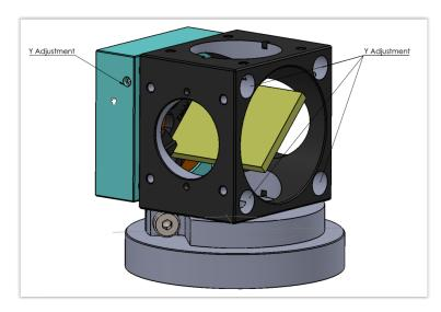
Figure 6.34: BFP detector mounting block with lateral adjustment screws
