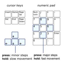
Figure 5.13: Stage movement using the keyboard
