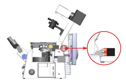
Figure 1.4: Illumination pillar interlock
